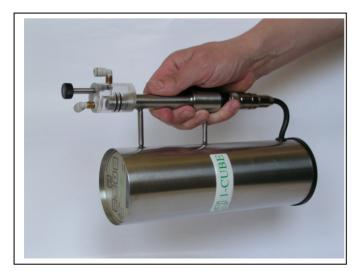
Whether your samples are soft drinks, mineral water or beer, with its measuring range from 0 ppm O2 to 10 ppm O2 the portable oxygen meter OXI is always the best option. The oxygen content is displayed in less than 2 minutes and is automatically transferred to the data memory.
