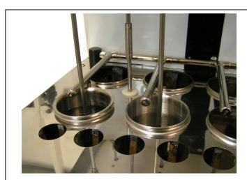
Details of jets for automatic distilled water refilling
