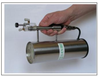
Whether your samples are soft drinks, mineral water or beer, with its measuring range from 0 ppb O2 to 10 000 ppb O2 the portable oxygen meter OXI is always the best option. The oxygen content is displayed in less than 2 minutes and is automatically transferred to the data memory.
