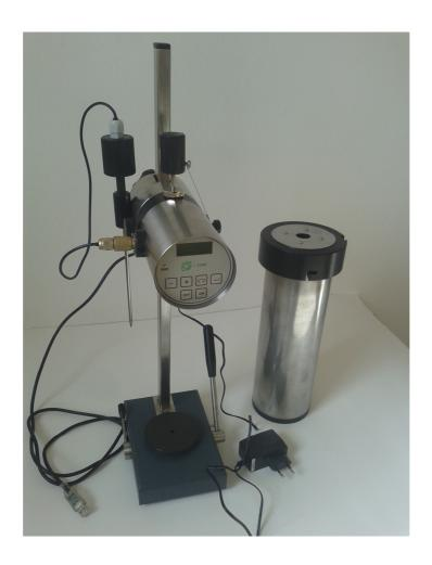
The instrument consists of a device stand, a protective container with cover, a lifting mechanism, a piercing needle, a microcomputer with keyboard and display, pressure and temperature sensors, USB cable for data transfer to PC and software for PC.
