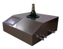
The hazemeter/color MZN based on the light scattering technique is used to detect the haze particles present in monitored liquid. The light coming from the source is focused by the system of apertures and lenses into a narrow beam entering a sample. A part of the beam is scattered around by haze
