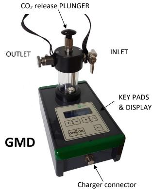
If the instrument is new or has not been used recently first check the battery charge. Press the ON key pad, hold for a second until the display illuminates. Then Press F1 (BATTERY) to display the voltage (see above). If necessary, recharge the instrument (see Recharging below)
