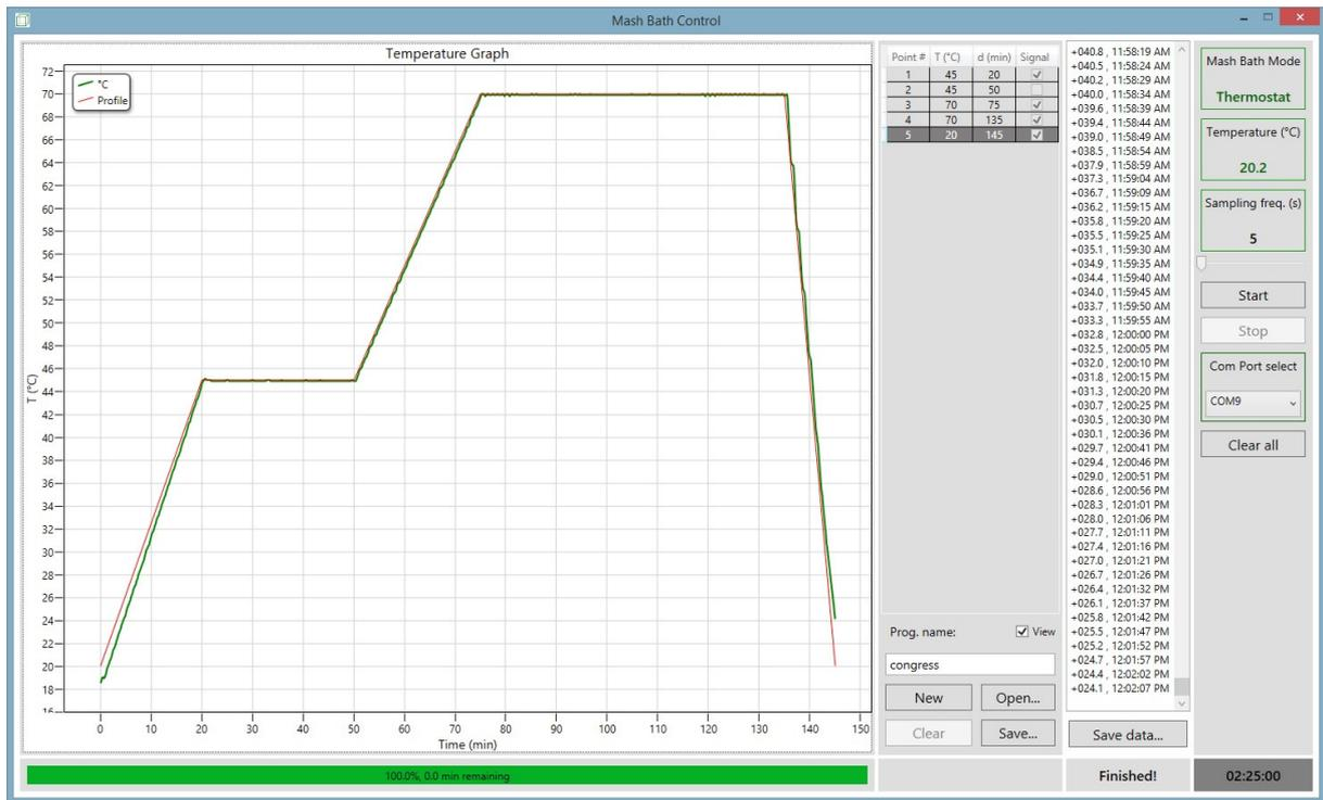
Monitoring software for Mash Bath equipped with a interface RS232-USB which allows the user to program temperature curve according to their needs in PC.
