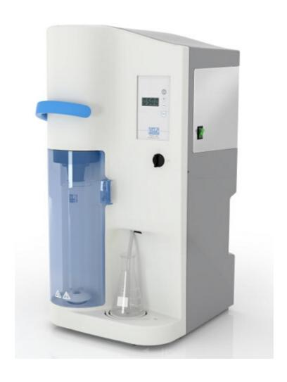
The UDK 129 runs automatically, after setting sodium hydroxide addition and distillation time using the LCD display in order to get reliable and accurate results. The high-precision pumps ensure constant accurate dosing of reagents and the cooling water is automatically stopped during pauses, thus cutting down on its consumption.
