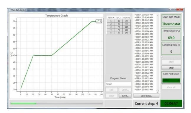
Software Monitoring allows the user to program temperature curve according to their needs in PC.
