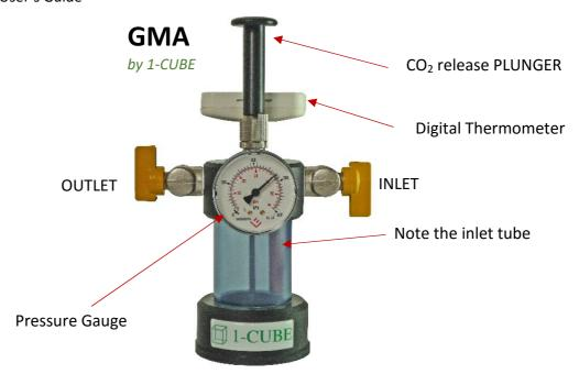
To start measuring the dissolved CO<sub>2</sub> in a sample, **first take a sample from a tank** as follows:
