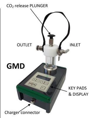
If the instrument is new or has not been used recently first check the battery charge. Press the ON key pad, hold for a second until the display illuminates. Then Press F1 (BATTERY) to display the voltage (see above). If necessary, recharge the instrument (see Recharging below)
