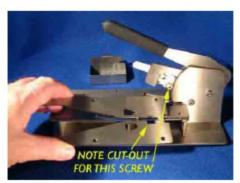
Slide the top plate into alignment with the other plates and drop the 6 screws back into position. Screw the 6 fixings in about 2 turns each to ensure full alignment of all plates and then fully tighten all screws.
