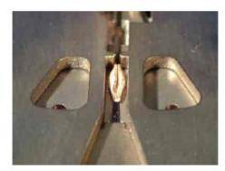
To achieve good splitting it is desirable that the germ end of the grain is slid into the small slot in the end stop. This guarantees the germ is centrally split even if the rest of the grain is not aligned properly. Experience has shown that the "V" shaped clamp will usually pull the grain into good alignment and symmetrical splitting will occur even if the germ end is not against the end stop.
