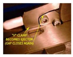
Further pressure on the operating lever opens the shutters and allows the sprung loaded "V" clamp to pass through the shutters, thus acting as an ejector to send the split grain into the two collecting trays.
