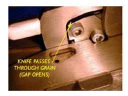
Phase two occurs as the knife passes right through the grain whilst it is still clamped. The handle then experiences distinct resistance as the "tooth" cam engages with the shutters.
