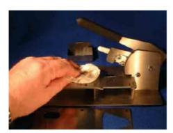
Remove the shim plate and wipe it clean. Note the shim plate is not stainless and some additives in certain oils may cause staining.
