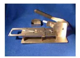
Slide the top plate off and wipe any oil from the underside
