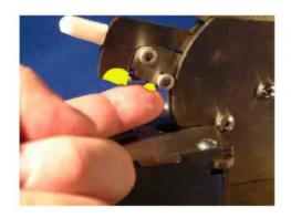
Apply a film of oil to both faces of the "tooth" and then apply a smear to each face of the "V" clamp. Note! Too much oil on the face of the "V" clamp will transfer to the shutters and could contaminate the sample. So, make sure it is just a film by wiping away the excess with a clean finger or a paper wipe. An invisible film will remain but this is adequate to ensure smooth operation.
