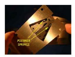
After cleaning, reassemble the shutter plate, making sure that the polymer springs are in the correct slot and pushed flush/sub-flush to the surface. Assemble and align it on top of the shim plate.
