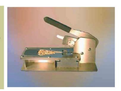
The Pneumac grain splitter has been designed to reliably and accurately split barley or wheat grains with the intention of exposing the germ in readiness for viability stain testing.
