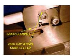
When the operating lever is pulled down there are three distinct phases to the cutting cycle which can be felt. The first resistance is felt when the "V" clamp aligns and locks the grain. At this point the knife has still not yet started cutting the grain.
