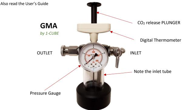
To start measuring the dissolved CO<sub>2</sub> in a sample, first take a sample from a tank as follows:
