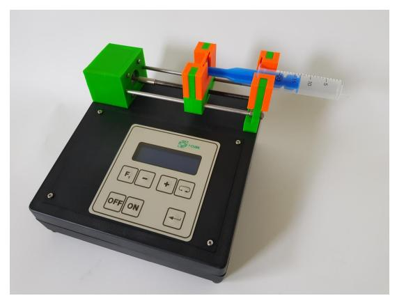
The 1-CUBE syringe pump is a programmable single channel infusion / withdrawal syringe pump. It has a plastic casing to provide stability, ensuring less vibration is transferred to the syringes. Setup is easy using the instruments keypad or via a computer with optional RS232/USB cable.
